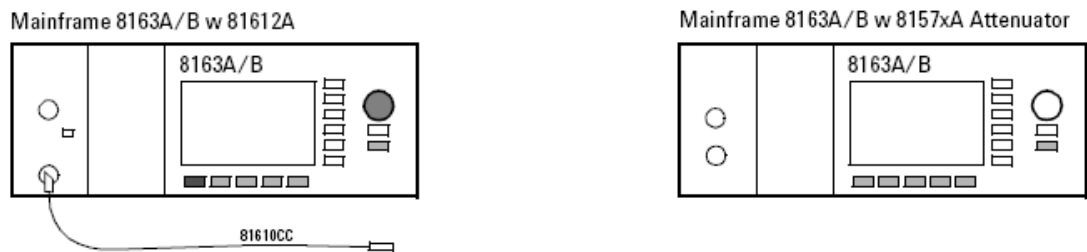
Figure 11 Return Loss Reference Setup for SM attenuators
